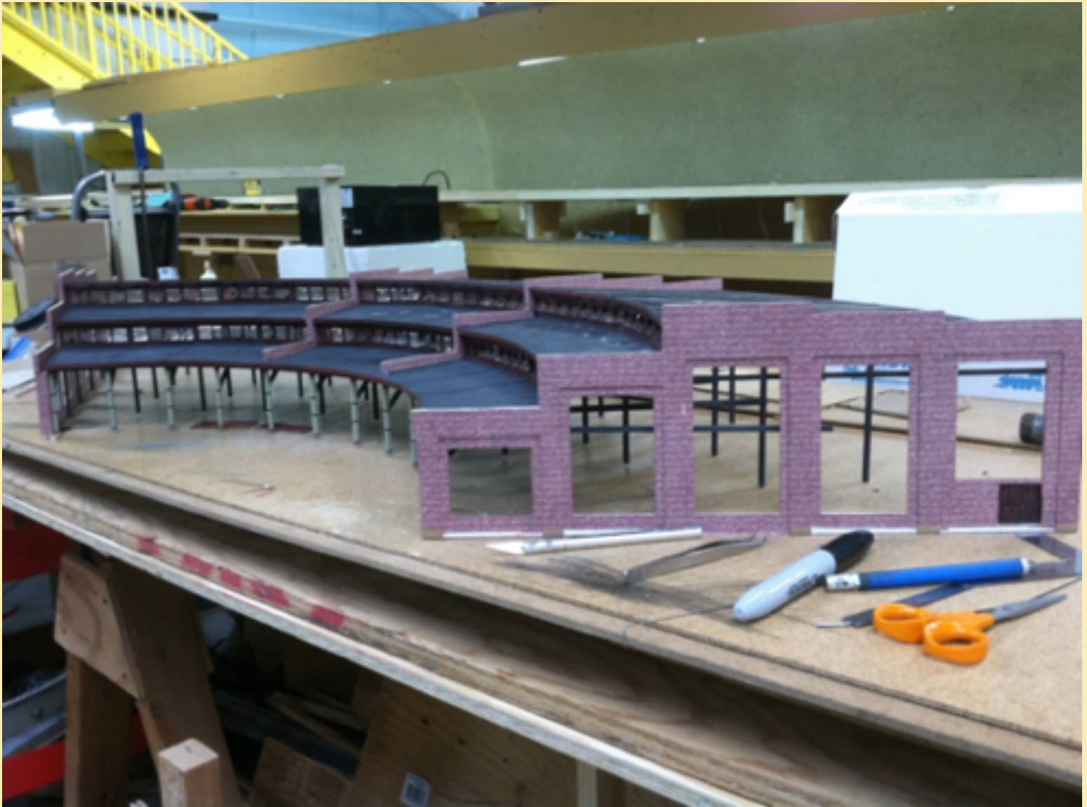
Figure 9. Completed walls ready for large windows.\
