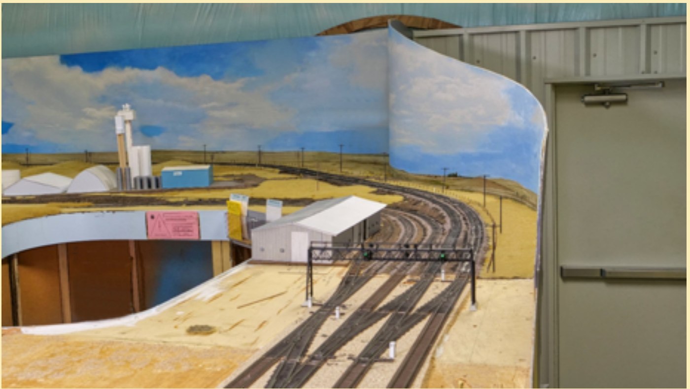
Figure 9. The east side of the Cheyenne signal bridge spanning 4 tracks at the west yard entrance of Cheyenne. Since no trains are on the block starting just past the signal bridge or on the following block, the two signals over each of the 2 departing tracks show green ABS aspects. The second track from the left is the beginning of the Harriman Cutoff (Track #3). The last track to the left is a stub track for the Cheyenne Stock Yard. The rear double doors to far right.
