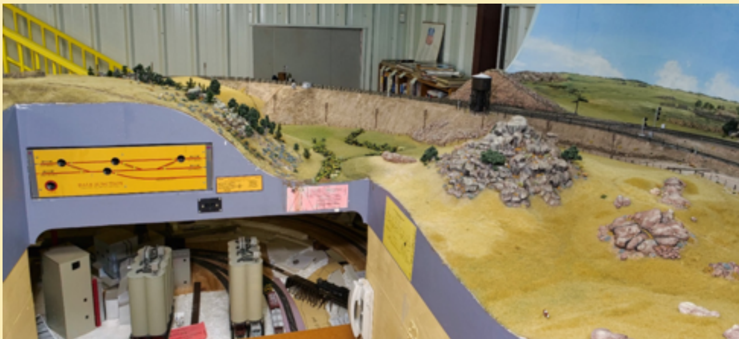
Figure 5. Tortoise machine switch Panel set in fascia at Dale. The scenery is complete here.
